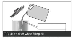
After installing the appropriate accessories for the selected installation method, remove the oil reservoir lid and fill the reservoir with oil to the 480ml level.
