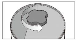
Turn the hand knob counter clockwise 1~2 turns before closing the lid to open the vent and relieve vacuum pressure.
