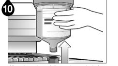
When the selected dispensing period of the Pulsarlube V has completed, remove the lubricator from the application.
