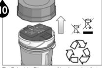
The Pulsarlube E is an eco-friendly product that can be disposed of separately. Turn the housing cap counterclockwise to disassemble the product for proper disposal.
